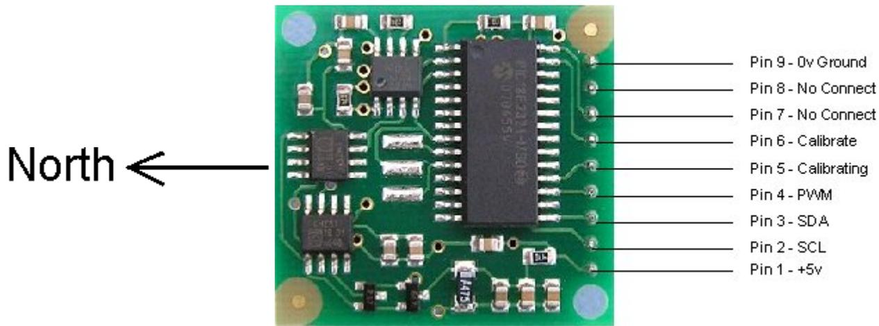
Before calibrating the compass, you must know **exactly** which direction is North, East, South and West. Remember these are the magnet poles, not the geographic poles. Don't guess at it. Get a magnetic needle compass and check it. When calibrating, make sure the compass is horizontal at all times with components upwards, don't tilt it. Keep all magnetic and ferrous materials away from the compass during calibration - including your wristwatch.
