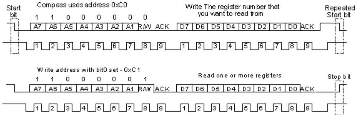
First send a start bit, the module address (0XC0) with the read/write bit low, then the register number you wish to read. This is followed by a repeated start and the module address again with the read/write bit high (0XC1). You now read one or two bytes for 8bit or 16bit registers respectively. 16bit registers are read high byte first. The compass has a 16 byte array of registers, some of which double up as 16 bit registers as follows;
