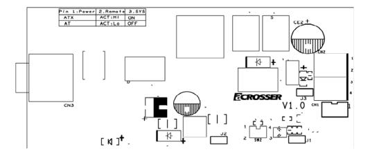
CN1: +5V stand by power supply and main power on/off trigger singal
