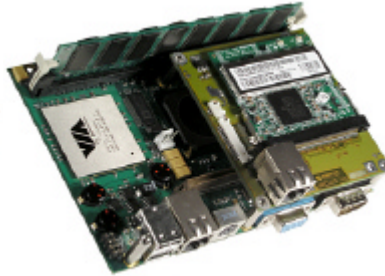
JREx-VE, no cooler JFLEX-MiniPCI-II WLAN card mounted SDRAM-DIMM mounted
