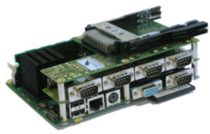
JREx-VE 300 JFLEX-SERIALGPIO1 JFLEX-PCMCIA1 SDRAM-DIMM mounted CompactFlash mounted
