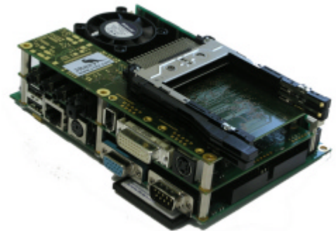
JREx-VE 300 JFLEX-Multimedia1 JFLEX-PCMCIA1 SDRAM-DIMM mounted CompactFlash mounted
